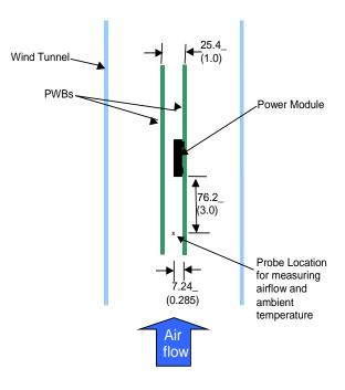
Figure 33. Thermal Test Set-up.
