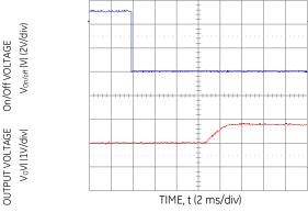
Figure 17 Typical Start-Up using Remote On/off with Prebias (Vin = 3.3Vdc, Vo = 1.8Vdc, Vo = 1.8Vdc, Vo = 1.8Vdc).
