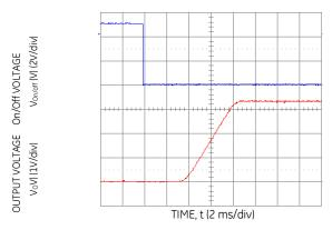
Figure 15. Typical Start-Up Using Remote On/Off with Low-ESR external capacitors (7x150uF Polymer) (Vin = 5Vdc, Vo = 3.3Vdc, Io = 5.0A, Co = 1050µF).
