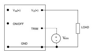
Figure 30. Circuit Configuration for programming Output voltage using external voltage source
