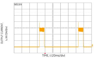
Figure 18. Output short circuit Current (Vin = 5Vdc, Vo = 0.75Vdc).
