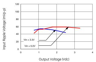
Figure 27. Input ripple voltage for various output with 2x150  $\mu F$  polymer and 2x47  $\mu F$  ceramic capacitors at the input (full load)
