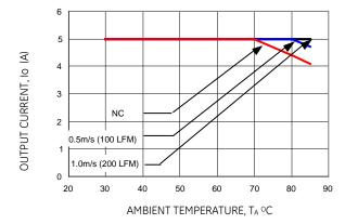
Figure 20. Derating Output Current versus Local Ambient Temperature and Airflow (Vin = 5.0Vdc, Vo=0.75 Vdc).
