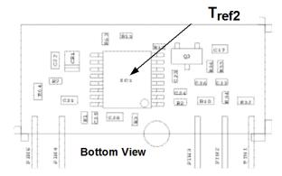
Figure 32. Tref Temperature measurement location.
