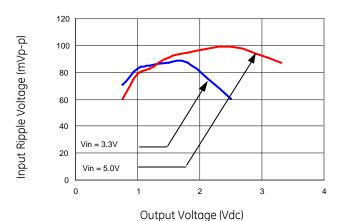
Figure 26. Input ripple voltage for various output with 1x150  $\mu$ F polymer and 1x47  $\mu$ F ceramic capacitors at the input (full load)
