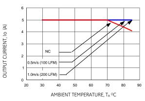
Figure 22. Derating Output Current versus Local Ambient Temperature and Airflow (Vin = 3.3Vdc, Vo=0.75 Vdc).
