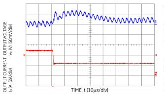
Figure 13. Transient Response to Dynamic Load Change from 100% of 50% full load (Vo = 3.3 Vdc, Cext =  $2x150~\mu F$  Polymer Capacitors).
