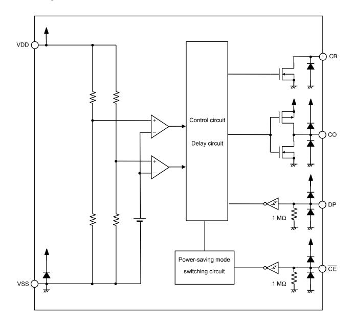
**\*1.** All diodes shown in the figure are parasitic diodes.
