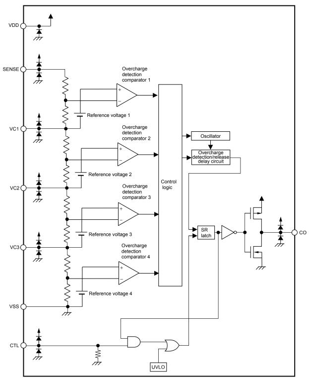
**Remark** The diodes in the figure are parasitic diodes.
