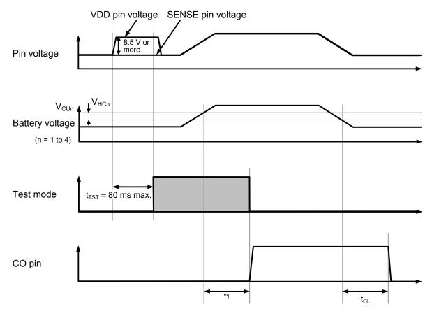
\*1. In the product  $t_{\text{CU}}$  = 4 s Typ. during normal mode,  $t_{\text{CU}}$  = 64 ms Typ. In the product  $t_{\text{CU}}$  = 2 s Typ. during normal mode,  $t_{\text{CU}}$  = 32 ms Typ. In the product  $t_{\text{CU}}$  = 5.65 s Typ. during normal mode,  $t_{\text{CU}}$  = 88 ms Typ.
