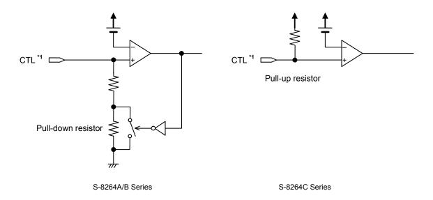
\*1. The reverse voltage "H" to "L" or "L" to "H" of CTL pin is VDD pin voltage – 2.8 V (Typ.), does not have the hysteresis.
