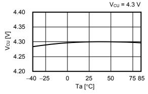
(2) Overcharge Release Voltage vs. Temperature
