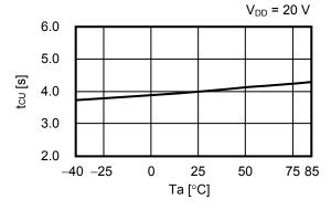
(2) Overcharge Release Delay Time vs. Temperature
