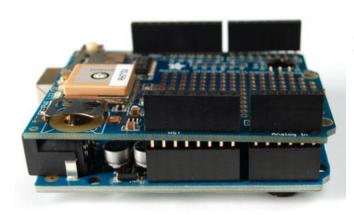
Fit the long pins through the pads until they slot into the Arduino. Depending on which version/type of Arduino you may need to use  $2 \times 8pin$  and  $2 \times 6pin$  or  $1 \times 10pin$ ,  $2 \times 8pin$  and  $1 \times 6pin$ .
