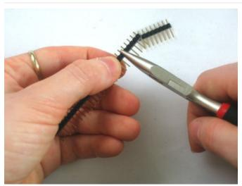
If you want to go with male headers, break off the 36-pin long stick into either  $2 \times 8pin$  and  $2 \times 6pin$  or  $1 \times 10pin$ ,  $2 \times 8pin$  and  $1 \times 6pin$  (depending on how many headers your Arduino has and which version it is)
