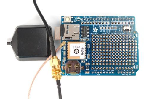
Active antennas draw current, so they do provide more gain but at a power cost. Check the antenna datasheet for exactly how much current they draw - its usually around 10-20mA. (http://adafru.it/960)
