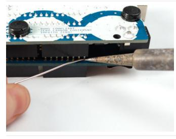
Turn the Arduino upside down so its resting on the long parts of the stacky headers and solder them from below.
