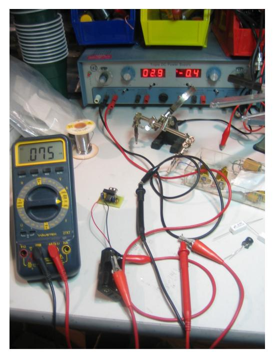
That means that the self-discharge rate is  $^{2}2000$  mAh / 0.1mA = 20,000 hours, more than 2 years. Most batteries don't last that long! Therefore we don't need a switch, when nothing is plugged in, almost no power is being used.
