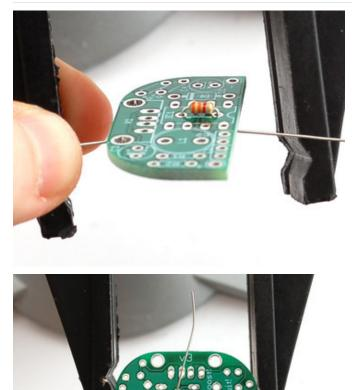
Bend the resistor into a staple and slip it onto the top of the Printed Circuit Board. Bend the little leads out so that you can flip over the PCB and the resistor will stay in place.
