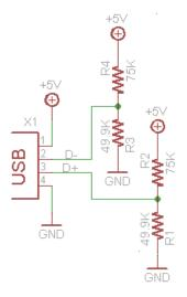
This time both voltages on the data lines are = 49.9K / (49.9K + 75K) \* 5.0V = 2.0V
