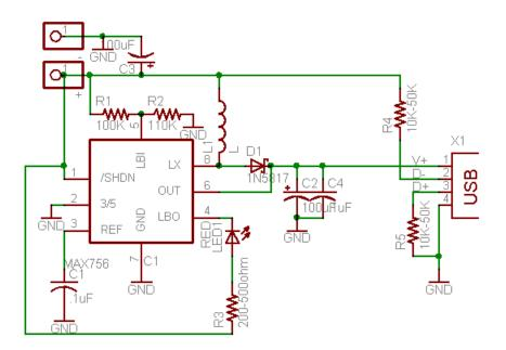
Note that because the mintyboost runs from 2 AA batteries, we can get 3V directly from the batteries so we connected the pullup right to the battery input.
