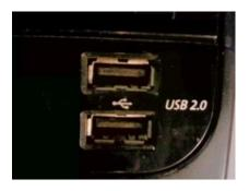
Every computer has a USB connector on it, and all the connectors are the same, with 4 pins. One pin is Ground, two pins are Data (D+ and D-) and the last pin is 5V power. The Ground and 5V pins are used to provide power to whatever is plugged in - keyboard, mouse, USB key, etc. The two data lines are used to transfer information back and forth - what keys are pressed, saving files to the USB drive, etc.
