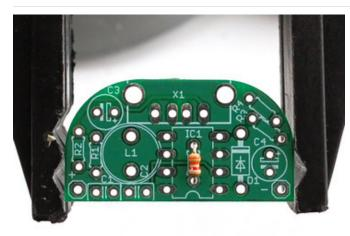
The first part we will place is the resistor **R5** - this is a small oval tan thing with two wires (leads) and color stripes. The stripes are orange orange red which indicates a 3.3K resistor. This resistor is used to improve the high current capability of the boost converter chip and is a new addition to the mintyboost. The resistor goes right in the middle, over the silkscreen text that says **R5**.
