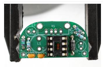
Next is the IC socket. This protects the chip and allows you to replace it if there are any problems. The socket goes *over* the 3.3K resistor but the resistor should not interfere as long as it was soldered in properly.
