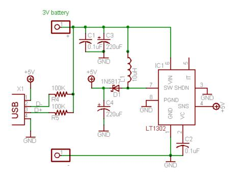
Smartphones started coming out and becoming popular, and devices with massive batteries, which meant that charging at 100mA was a no go. The mintyboost was then upgraded to the LT1302 (https://adafru.it/c3U), a more expensive chip but one with a nice 500mA output ability!
