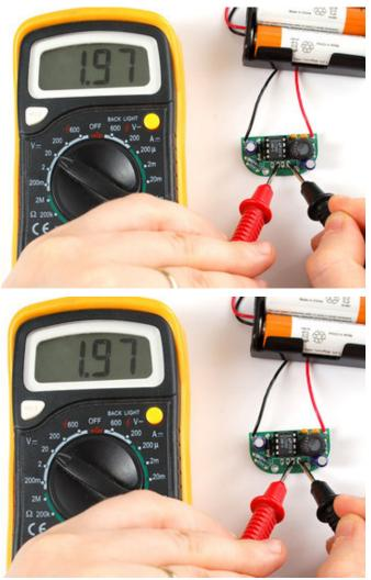
Next check between the rightmost pin and the second and third pin. They should both be at just about 2.0V
