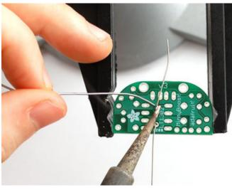
Now you'll solder! Place the flat of the soldering iron tip against the silver ring (pad) and one of the wires of the resistor (lead) at the same time for 2 seconds. This will heat them both up to 600-700 degrees. Then poke the end of the solder so that it flows into the hole and forms a solder joint.
