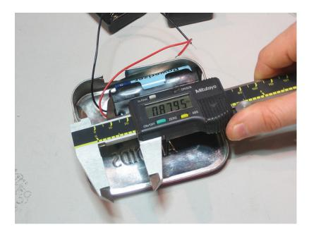
I also try out another battery holder I have, this gives me more space, 1.25"x0.85"...but the batteries go in sideways so one would have to remove the holder to change the batteries. I'd prefer that you can just take them out directly, so I don't go with this one (it also turns out I don't need that extra space).
