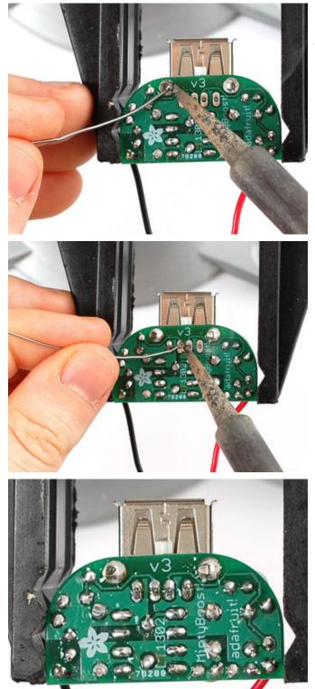
The two large side connectors are used for mechanical strength. They keep the connector attached solidly to the PCB so make sure to use lots of solder or it will break off from use.
