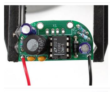
Finally, carefully insert the boost converter chip. Make sure the notch in the chip matches the notch in the socket. If the socket was inserted backwards, make sure the notch faces the flat edge of the PCB as shown. Make sure the chip is seated all the way in and that the pins aren't bent.
