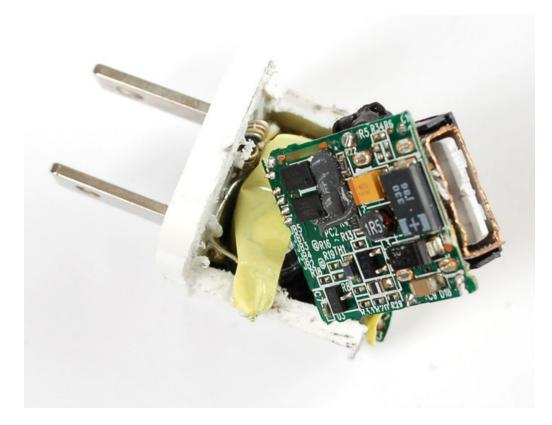
Taking it apart, desoldering the 4 data line resistors and measuring them on our multimeter, we found the following as shown in the schematic:
