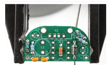
The next type of part we'll place is the ceramic capacitor. These are parts **C1** and **C2**. Ceramic capacitors have a nice property that they are symmetric/non-polarized. That means they can go in 'either way'. Place the capacitor so that the 2 legs (leads) slide thru the two metal holes in the PCB (pads). The capacitor will sit flat against the PCB.
