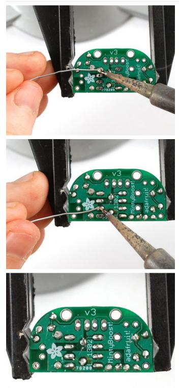
The socket has short legs so it can be annoying to keep in the right position. Hold it in place with one finger and 'tack solder' a corner.
