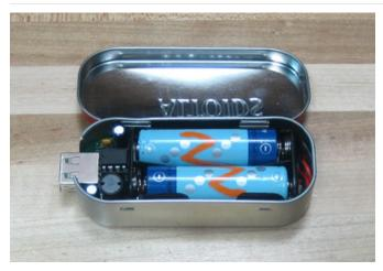
You're done! Remember that because the boost chip uses virtually no power, you dont have to remove the batteries to turn off the MintyBoost. Just plug and unplug devices whenever you want.
