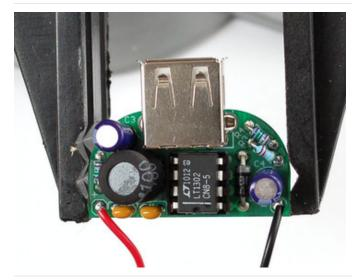
Next is the USB type A connector. This is the connector that is on a computer, and nearly all USB charging cables will plug into it. The Connector should snap easily in place.
