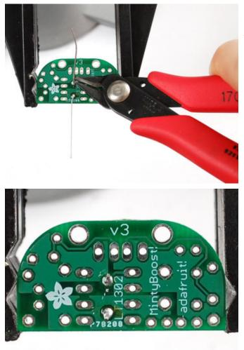
Now we will get rid of all that excess wire. Use your diagonal nippers to clip the wire just above the end of the solder joint. There should be almost no 'wire' sticking out.
