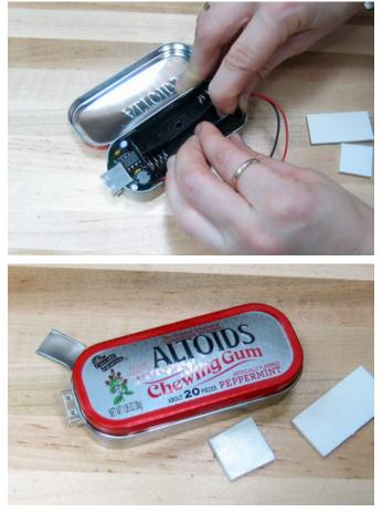
Try a test fit. Slide the board in first, then fit the battery pack in. Don't put the batteries in for this test! The circuit board could short against the tin and destroy the circuit!
