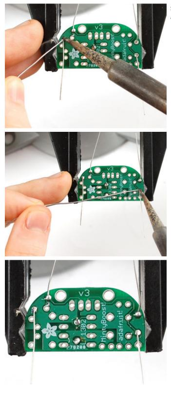
Solder the resistors as you did the 3.3K one, one point at a time, checking your work.
