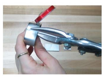
Cut two notches in the end of the tin, just about where the flat part ends and the tin starts to round out.
