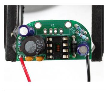
Next, solder in the 2xAA battery holder. The red wire goes to the hole marked + and the black wire goes to the hole marked -.
