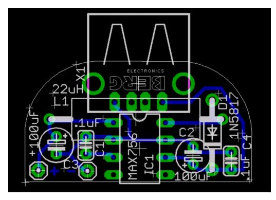
Since I am know this is just a prototype version, I make the PCB single sided -- for easy etching. I also make the traces really large.
