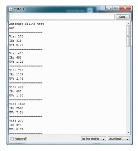
In this screenshot I pointed a UV LED onto the sensor to simulate a really high UV index of 7. Indoors, expect to get a UV index of well below 1. Even glass windows are excellent at filtering UV light so if you want to measure the actual UV outside point the sensor right at the sun!
