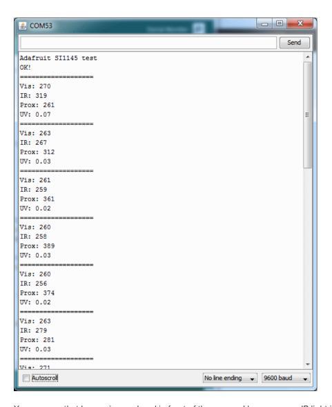
You can see that by moving my hand in front of the sensor, I bounce more IR light into the proximity sensor and the value goes from 261 up to 361
