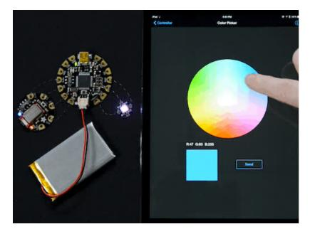
For advanced hackers, they'll be very happy to use the standard Nordic UART RX/TX connection profile. In this profile, the Bluefruit acts as a data pipe, that can 'transparently' transmit back and forth from your iOS or Android device. You
