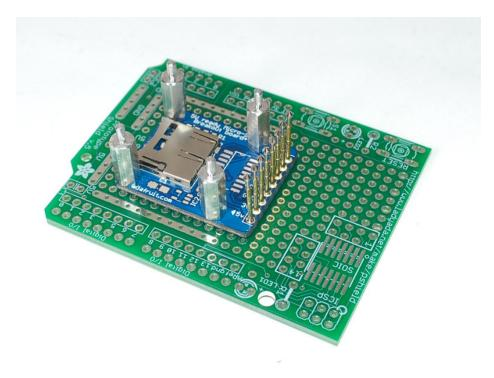
Mark and drill the mounting holes - four in this case. Luckily (or on purpose???) I placed the mounting holes on 0.1" boundaries.
