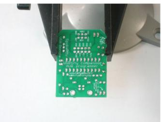
Next up are the 2 47 ohm resistors. Place them as shown. Bend the legs out, flip the PCB, solder the 4 joints and clip them.
