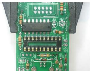
Next to be placed is the 74AHC125 buffer. This chip does a level-shifting conversion on signals from the USBtiny microcontroller to the device being programmed. This way you can safely program chips that vary from 1.8V to 5.5V voltage.
