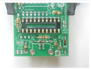
Next is the socket for the microcontroller that does all the hard work. A socket is useful because you can replace the chip in case of upgrade or damage. Sockets have a little notch in them to indicate which way to put in the chip. This notch should match the notch in the silkscreen image, in this picture, the notch is on the left-hand side.
