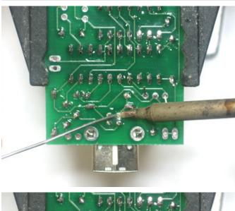
Solder in the three-pins of the oscillator and all 6 pins of the USB connector. Make sure to not bridge any of the square-pins and put plenty of solder on the mechanical tabs. These provide the resistance when you plug in a cable so it's important that they are soldered well, as shown here.
