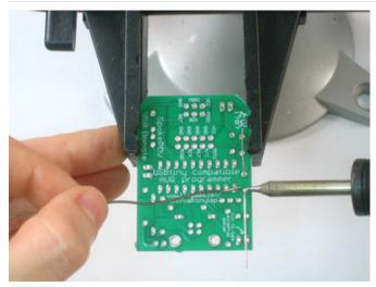
Solder the legs. Hold the tip of iron against the wire leg and the metal ring at the same time, after 2 counts, poke the solder in till it creates a nice pool. Then remove the solder, wait a half count, then remove the iron. Do this for both legs.
