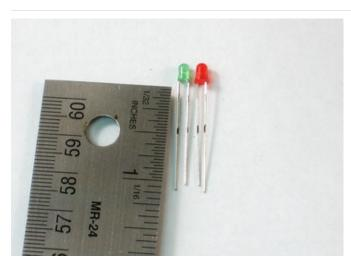
The two LEDs are next. They should stand-off a bit from the PCB so make a marking about 1/2" (1cm) from where the colored plastic ends.
