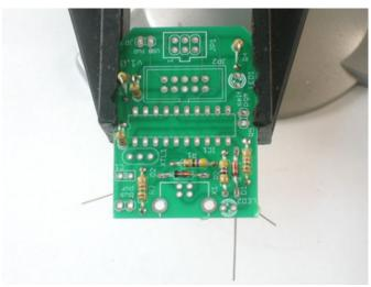
Next are the zener diodes. Diodes are directional so make sure to put them in as shown. There's a white stripe on the PCB drawing that matches the black stipe on the glass diode.
