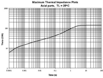
FIGURE 7. Thermal impedance (axial leads).
