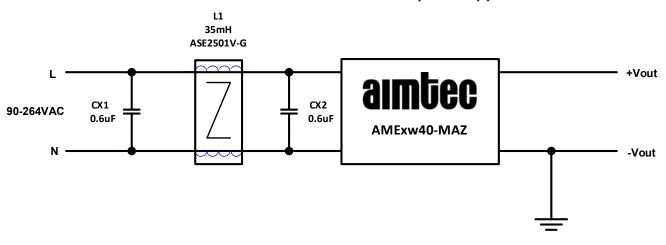
The Application circuit is EMC compliant for any type of Earth/Ground connection: Input Ground connection, Output Ground connection as shown or both sides, which is not recommended if the product Isolation is used as a Safety feature.
