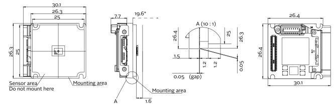
\*Mechanical length for C-Mount, for other mounts and details, see the user guide.
