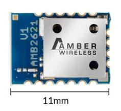
The AMB2621 is an ultra-low power 2.4 GHz wireless module integrating the nRF52832 System on Chip including a 2.4 GHz transceiver and an ARM Cortex<sup>™</sup>-M4F CPU with flash memory. The module is optimized for applications where costs and low-power optimization really matter. Several pins with alternate functions are available to e.g. connect LEDs, or realize an SPI, I2C, ADC or handshake for the UART as well as NFC.
