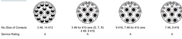
The following RADSOK layouts incorporate RADSOK sockets in sizes 12, 8, 4, and 0, with standard contacts in size 16. All patterns are available in GT Series and Threaded 5015 Series. Only shell sizes 18-28 are available in P-Lok. Consult Amphenol Industrial, Fraser, MI for availability of P-Lok.
