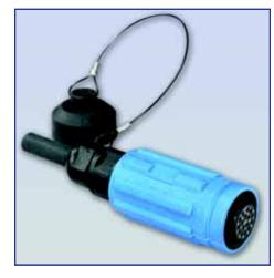
The Amphe-Y features RADSOK<sup>®</sup> sockets and is a high amperage/high voltage assembly designed for the rail industry. This product is used in mass transit traction motors and is an ideal replacement for high-current bolted connections that absorb high labor costs and add excessive time for maintenance and repair procedures.
