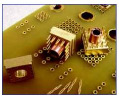
The RADSOK<sup>®</sup> PowerBlok<sup>™</sup> provides a high current single-point connection to the PCB with the proven reliability of compliant pin signals. The PowerBlok<sup>™</sup> is designed to bring up to 70 Amperes to the board, utilizing our custom 3.0mm RADSOK<sup>®</sup> design. The compliant pins are press-fit into the board to secure a solid connection and even flow.
