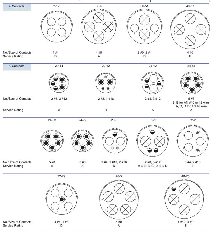
The following RADSOK layouts incorporate RADSOK sockets in sizes 12, 8, 4, and 0, with standard contacts in size 16. All patterns are available in GT Series and Threaded 5015 Series. Only shell sizes 18-28 are available in P-Lok. Consult Amphenol Industrial, Fraser, MI for availability of P-Lok.
