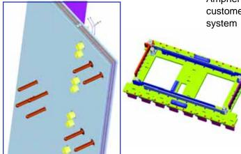
The RADSOK<sup>®</sup> PGY<sup>™</sup> is our orthogonal card edge series. The 5.7mm PGY<sup>™</sup> is our highest current board level product rated to 120 Amperes. The PGY<sup>™</sup> is connected to the board through a solder reflow process. The busbar pin will mate horizontally with RADSOK<sup>®</sup> slightly above the board.
