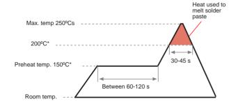
\* Melting point temp. depends on solder properties
