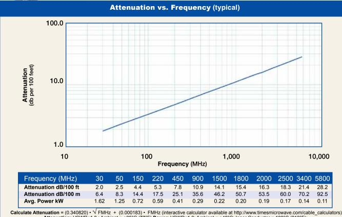
Calculate Attenuation = (0.340820) • √ FMHz + (0.000183) • FMHz (interactive calculator available at http://www.timesmicrowave.com/cable\_calculators)
