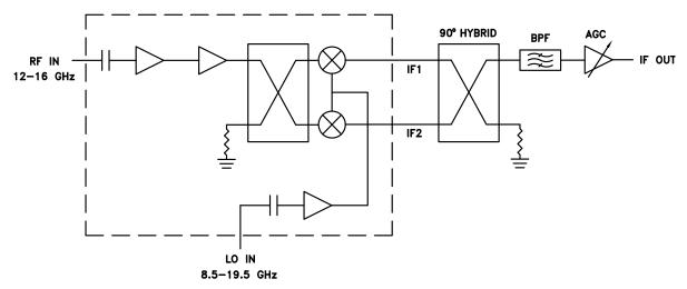
Note: LSB and USB is determined by GND on Hybrid
