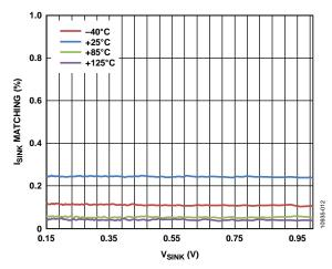
Figure 12. Typical Sink Current Matching vs. Sink Voltage,  $R_{SET} = 25.5 k\Omega$
