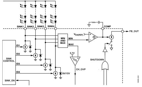
Figure 22. Error Amplifier Power Control
