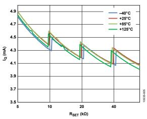
Figure 5. Typical Operating Current vs. R<sub>SET</sub>
