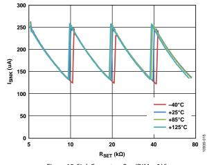
Figure 15. Sink Current vs.  $R_{SET}$  (DIM = 0 V)
