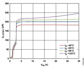
Figure 6. Typical Standby Current vs.  $V_{IN}$ , EN = 0 V
