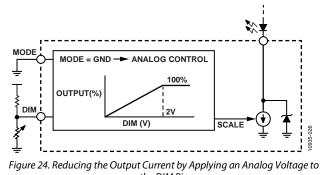
the DIM Pin If MODE is connected to REG or to a 52.3 k $\Omega$  resistor at startup, a PWM duty cycle applied to the DIM pin is internally filtered and used to scale the output currents. Set the DIM pin
