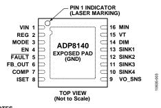
NOTES 1. CONNECT THE EXPOSED PAD OF THE LFCSP TO GROUND.
