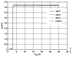
Figure 4. Typical Operating Current vs.  $V_{IN}$ , EN = 3 V,  $R_{SET} = 71.5 k\Omega$
