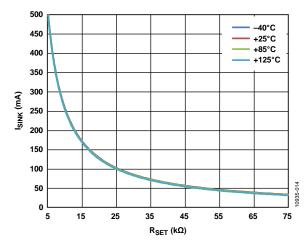
Figure 14. Sink Current vs.  $R_{SET}$  (DIM = 3 V)
