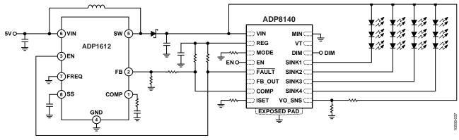
Figure 35. ADP8140 with a Boost Power Stage
