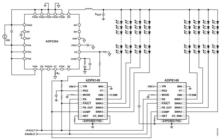
Figure 36. Multiple ADP8140 ICs with One Power Stage
