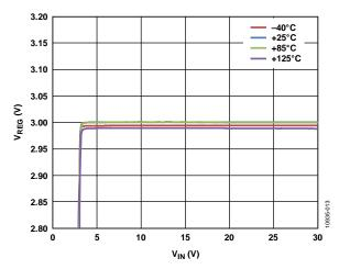
Figure 13. REG Voltage vs. Input Voltage
