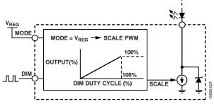
Figure 25. Reducing the Average Output Current by Pulse Width Modulating the Current Sinks with the DIM Pin
