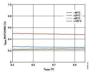
Figure 11. Typical Sink Current Matching vs. Sink Voltage,  $R_{SET} = 7.32 k\Omega$
