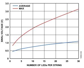
Figure 30. Voltage on SINKx Pins Given a Normal Distribution of  $V_{\rm F}$ , Standard Deviation = 70 mV
