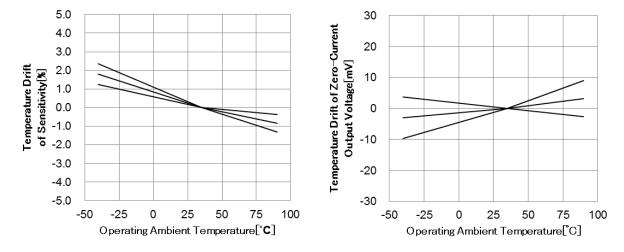
Figure 5. Temperature Drift of Sensitivity and Zero-current output Voltage.
