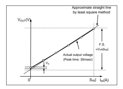
Figure 4. Output characteristics of CQ-330J
