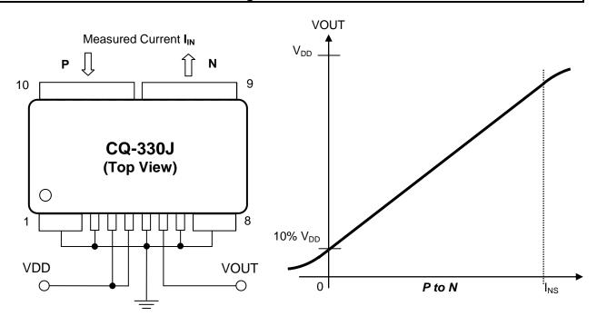
Figure 2. Pin assignment and typical output characteristics of CQ-330J
