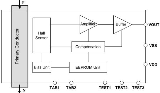
Figure 1. Functional block diagram of CQ-330J
