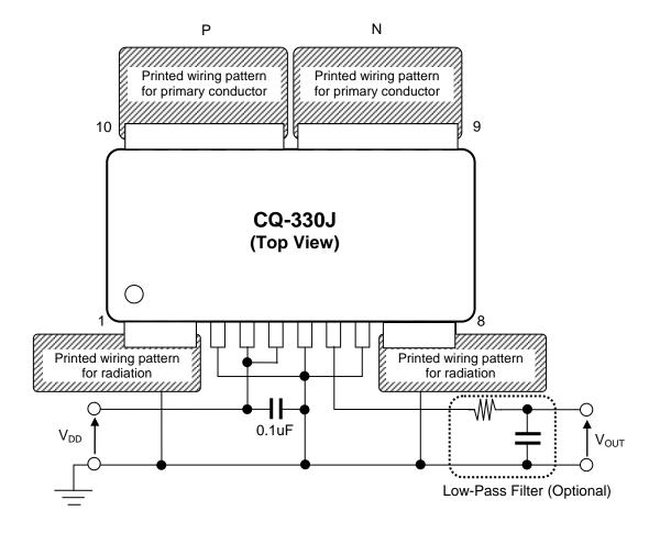
Figure 7. Recommended external circuits
