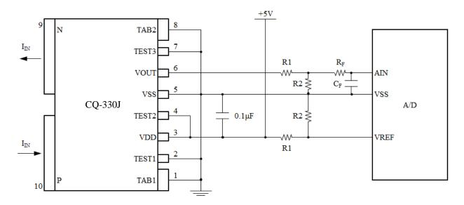
Figure 8. Recommended external circuits of CQ-330J
