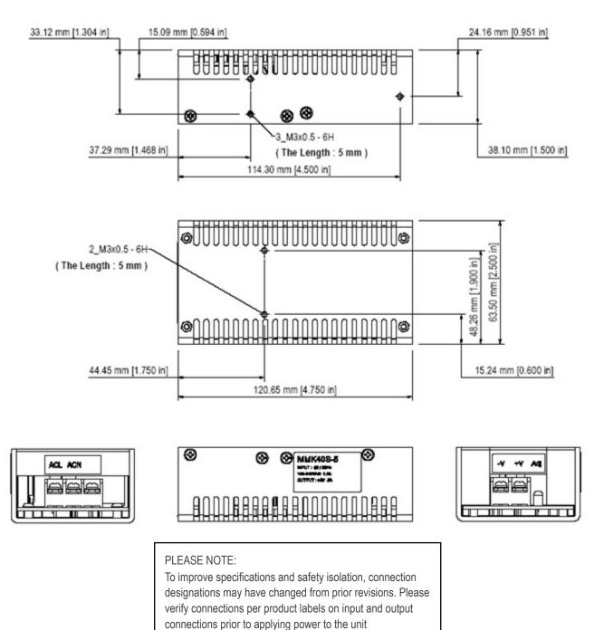
Note: For our M3 x 0.5 aluminum threaded holes: Recommended torque: 2.5 in-lbs, 3 in-lbs maximum (2.9 kgf-cm/3.5 kgf-cm max)
