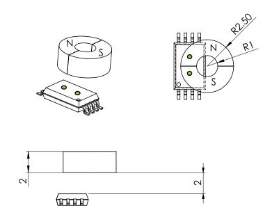
Figure 11-3 Magnet's postion relative to IC with on-axis orientation
