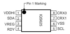
Figure 1-1 Pin out of IQS625 TSSOP (3X6.4)-8 package.
