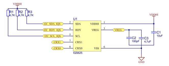
Figure 1-2 IQS625 reference schematic
