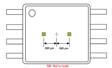
Figure 11-1 - Technical Drawing showing hall placement within the package. The Hall-Plates are shown as the two green pads and the center of the magnet is shown by the red cross.
