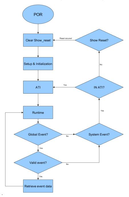
Figure 5-7 Master command structure and runtime event handling flow diagram
