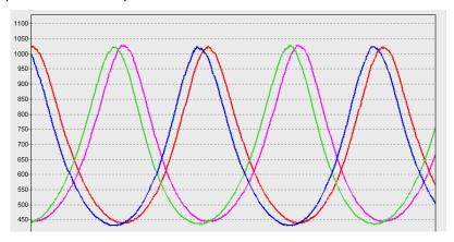
Experimentally, jog the XYZ alignment of the magnet relative to the IC and perform at least one full rotation of the magnet, assess the peaks of the channels; repeat this until all channels have approximately the same amplitude.
