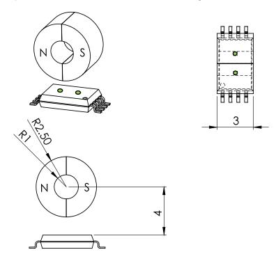
Figure 11-2 Magnet's postion reletave to IC with off-axis orientation
