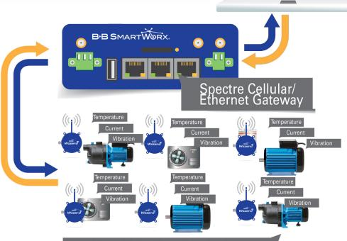
Wzzard™ Intelligent Edge Nodes/ Wireless SmartMesh IP Sensor Network
