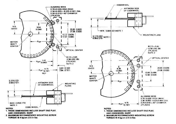
Figure 2. Mounting Plane Side A.
