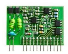
Thermocouple B (Pt30%Rh-Pt) input. Measuring range +100 to +1800°C. Accuracy  $\pm 0.3\%$  from reading +1.0°C from +300 to +1800°C. Linearized, without cold junction compensation. Galvanically unisolated.
