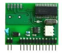
Input for measurement of frequency of contact switching 0 to 5kHz, resolution 1Hz, accuracy  $\pm (0.2\%$  from reading + 1Hz) maximum resistance of closed contact: 10 kohms minimum resistance of open contact: 250 kohms, minimum duration of input pulse: 30us, galvanically unisolated.
