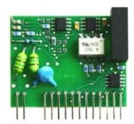
Accuracy  $\pm 0.1\%$  FS (± 20 mV). Galvanically isolated. Galvanic isolation is not designed as safety protection.
