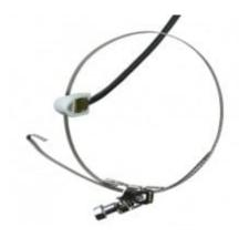
Temperature probe with Pt1000 sensor. Surface probe for tubing and flat surface, range from -30 to +130 $^{\circ}$ C, 2 meters cable, IP65. With CINCH connector.
