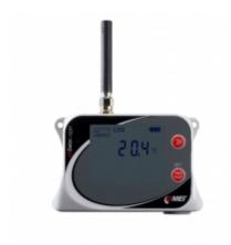
GSM datalogger is designed to record temperature. In case of exceeded set limits, SMS and JSON messages can be sent via GPRS data connection. Measured values can be sent to the internet storage <u>COMET Cloud</u>, which is a complete monitoring, alarm and analysis system.
