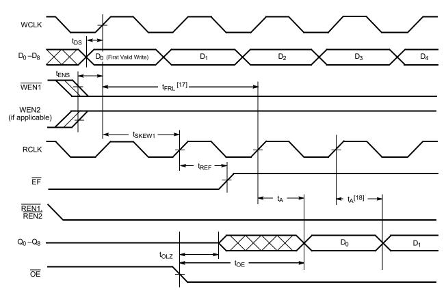
Notes 17. When t<sub>SKEW1</sub> ≥ minimum specification, t<sub>FRL</sub> (maximum) = t<sub>CLK</sub> + t<sub>SKEW2</sub>. When t<sub>SKEW1</sub> < minimum specification, t<sub>FRL</sub> (maximum) = either 2\*t<sub>CLK</sub> + t<sub>SKEW1</sub> or t<sub>CLK</sub> + t<sub>SKEW1</sub>. The Latency Timing applies only at the Empty Boundary (EF = LOW). 18. The first word is available the cycle after EF goes HIGH, always.
