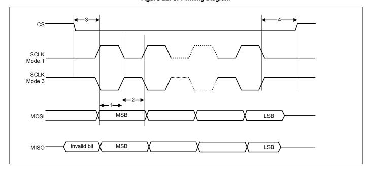
Figure 12. SPI Timing Diagram
