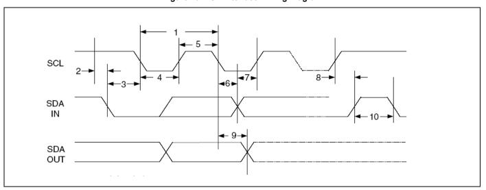
Figure 13. BSC Interface Timing Diagram
