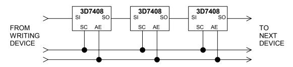
Figure 5: Cascading Multiple Devices
