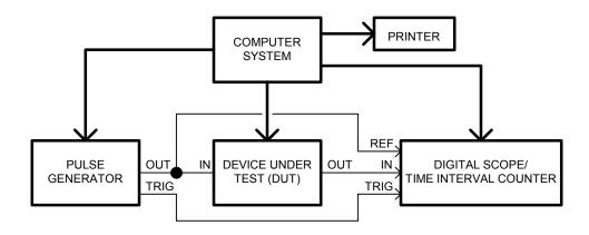
Figure 6: Test Setup
