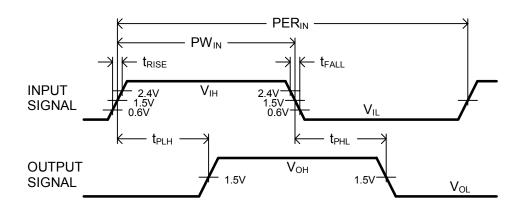
Figure 7: Timing Diagram
