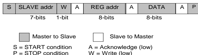
Figure 24: I 2 C Byte Write (SDA line)
