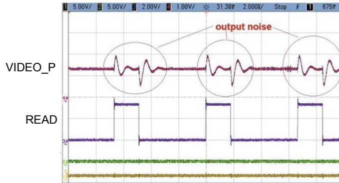
Figure 15: Bad READ signal coupling to the output by a ground loop
