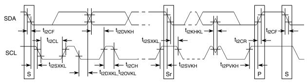
Figure 34. I<sup>2</sup>C Bus AC Timing Diagram
