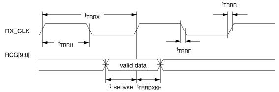
Figure 16. TBI Single-Clock Mode Receive AC Timing Diagram
