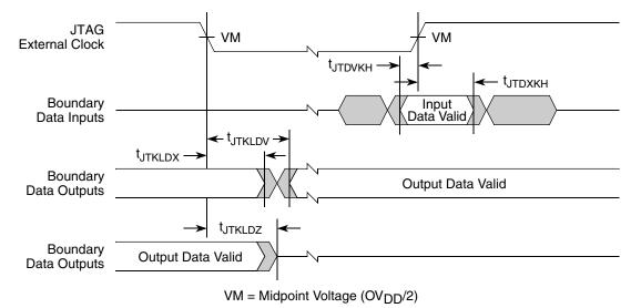
Figure 32. Boundary-Scan Timing Diagram
