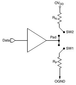
Figure 51. Driver Impedance Measurement
