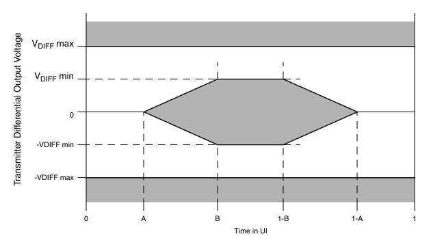
Figure 43. Transmitter Output Compliance Mask
