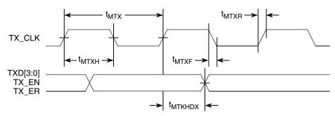
Figure 11. MII Transmit AC Timing Diagram
