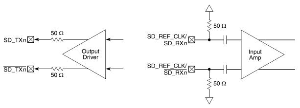
Figure 38. Driver and Receiver of SerDes (PCI Express, Serial RapidIO, and SD\_REF\_CLK/SD\_REF\_CLK
