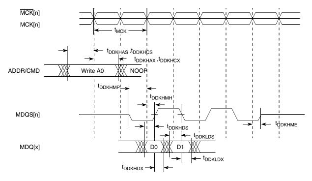
Figure 4. DDR SDRAM Output Timing Diagram
