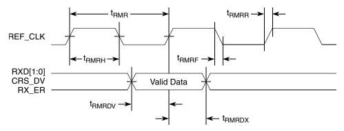
Figure 20. RMII Receive AC Timing Diagram
