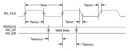
Figure 13. MII Receive AC Timing Diagram
