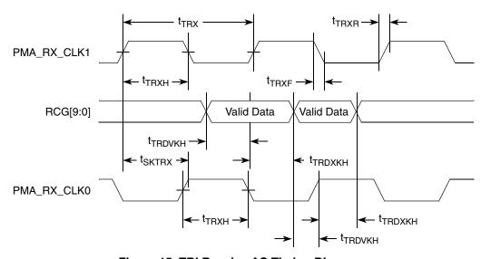
Figure 15. TBI Receive AC Timing Diagram
