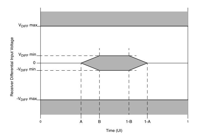
Figure 45. Receiver Input Compliance Mask
