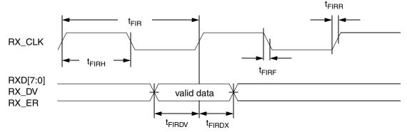
Figure 7. FIFO Receive AC Timing Diagram
