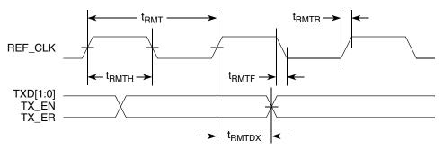
Figure 18. RMII Transmit AC Timing Diagram
