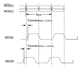
Figure 3. Timing Diagram for tDDKHMH
