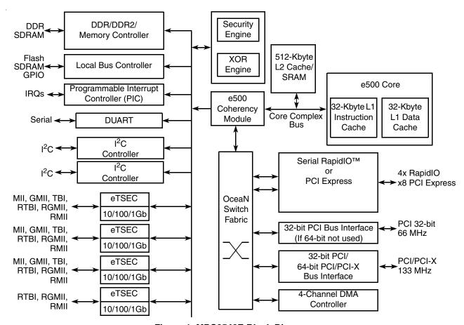
Figure 1. MPC8548E Block Diagram
