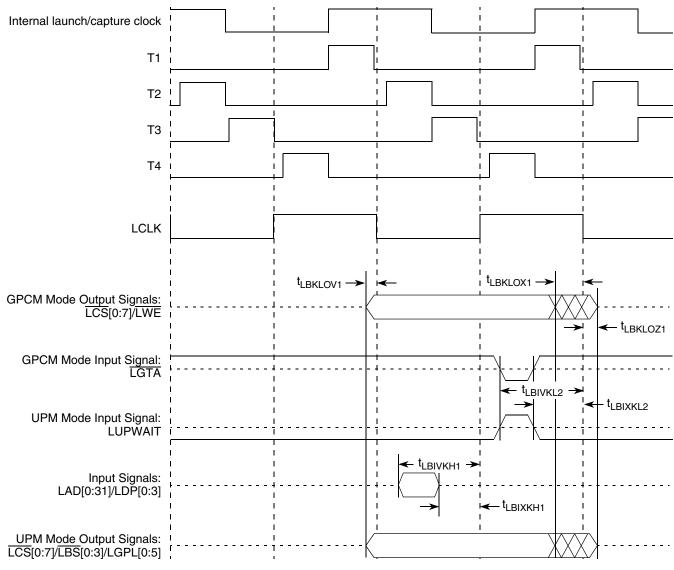
Figure 28. Local Bus Signals, GPCM/UPM Signals for LCCR[CLKDIV] = 8 or 16 (PLL Bypass Mode)
