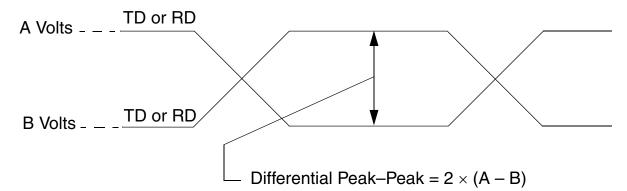
Figure 42. Differential Peak-Peak Voltage of Transmitter or Receiver
