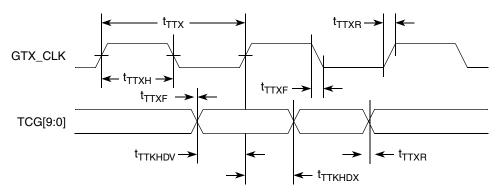
Figure 14. TBI Transmit AC Timing Diagram
