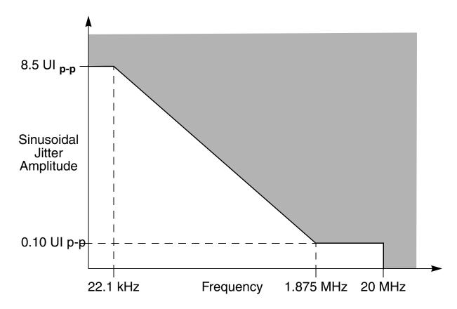
Figure 44. Single Frequency Sinusoidal Jitter Limits
