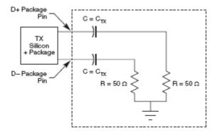
Figure 41. Compliance Test/Measurement Load
