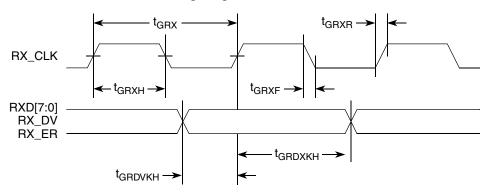
Figure 10. GMII Receive AC Timing Diagram
