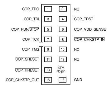
Figure 52. COP Connector Physical Pinout
