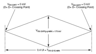
Figure 40. Minimum Receiver Eye Timing and Voltage Compliance Specification
