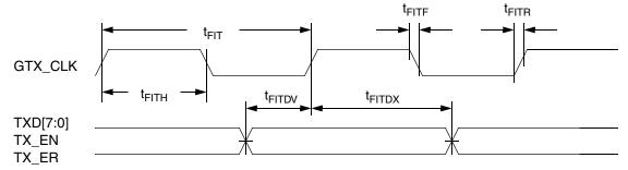
Figure 6. FIFO Transmit AC Timing Diagram
