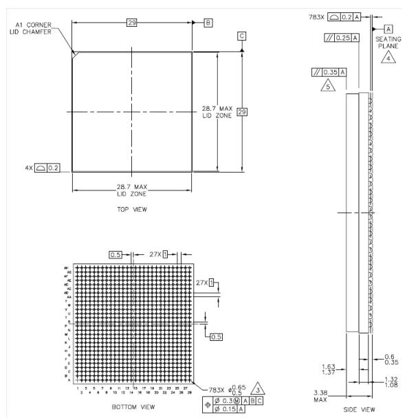
Figure 46. Mechanical Dimensions and Bottom Surface Nomenclature of the HiCTE FC-CBGA and FC-PBGA with Full Lid
