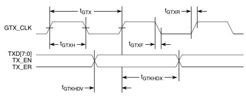
Figure 8. GMII Transmit AC Timing Diagram
