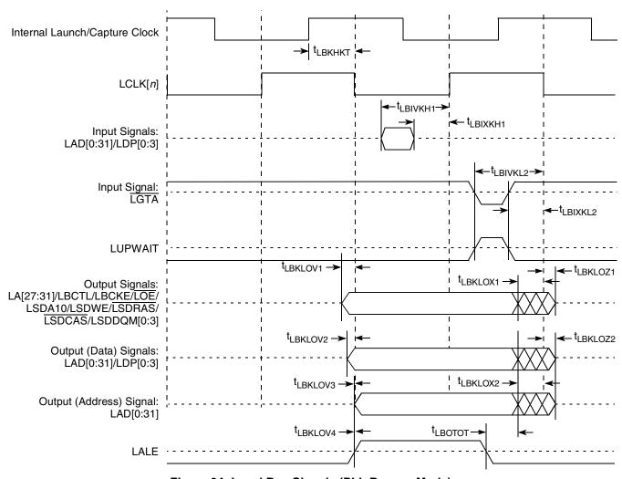
Figure 24. Local Bus Signals (PLL Bypass Mode)
