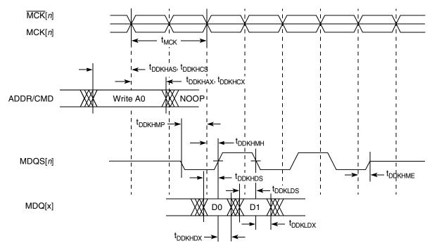
Figure 4. DDR SDRAM Output Timing Diagram
