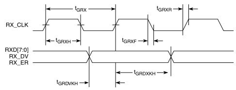
Figure 10. GMII Receive AC Timing Diagram
