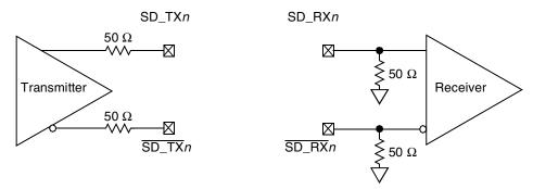
Figure 47. SerDes Transmitter and Receiver Reference Circuits
