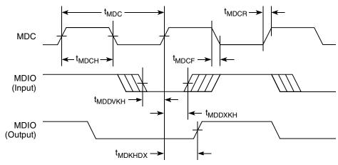
Figure 21. MII Management Interface Timing Diagram
