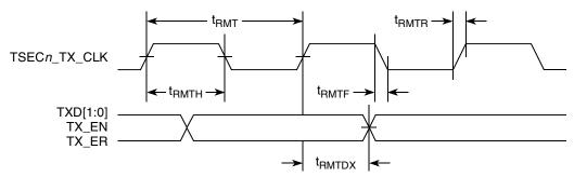
Figure 18. RMII Transmit AC Timing Diagram
