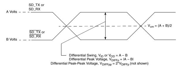
Figure 38. Differential Voltage Definitions for Transmitter or Receiver
