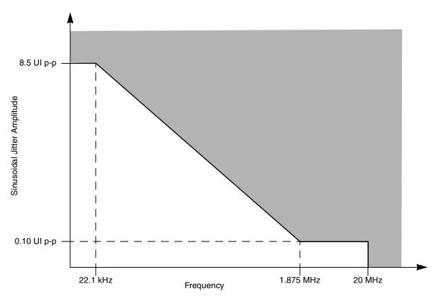
Figure 53. Single Frequency Sinusoidal Jitter Limits
