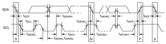
Figure 34. I<sup>2</sup>C Bus AC Timing Diagram
