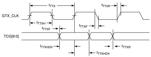
Figure 14. TBI Transmit AC Timing Diagram
