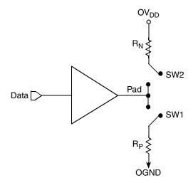
Figure 60. Driver Impedance Measurement
