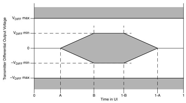
Figure 52. Transmitter Output Compliance Mask
