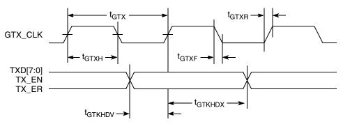
Figure 8. GMII Transmit AC Timing Diagram
