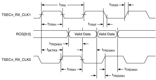
Figure 15. TBI Receive AC Timing Diagram
