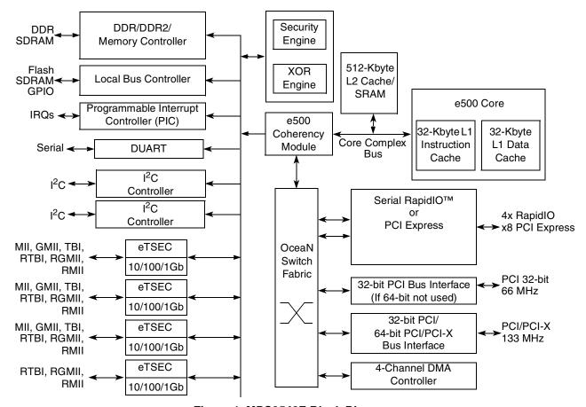
Figure 1. MPC8548E Block Diagram
