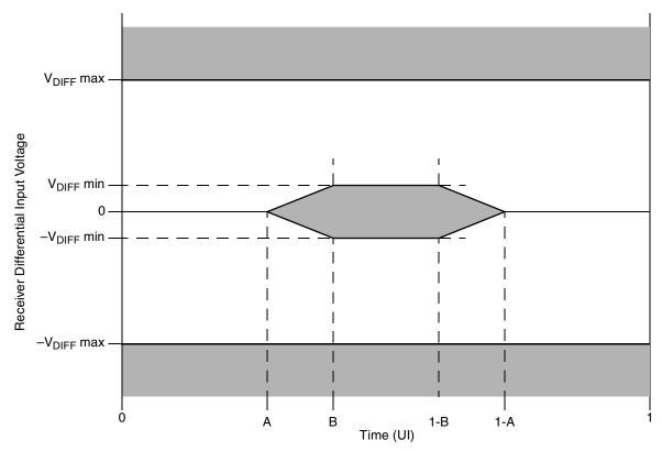
Figure 54. Receiver Input Compliance Mask
