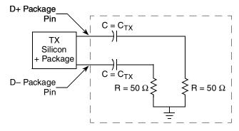
Figure 50. Compliance Test/Measurement Load
