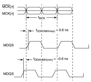
Figure 3. Timing Diagram for tDDKHMH
