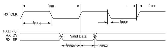
Figure 7. FIFO Receive AC Timing Diagram
