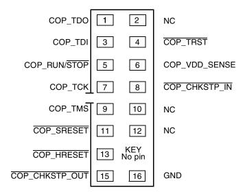
Figure 61. COP Connector Physical Pinout
