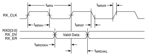
Figure 13. MII Receive AC Timing Diagram
