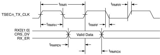
Figure 20. RMII Receive AC Timing Diagram
