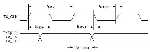
Figure 11. MII Transmit AC Timing Diagram
