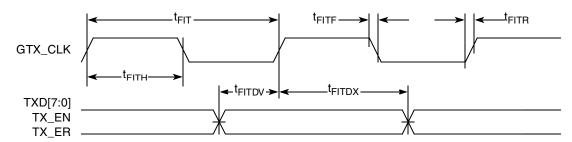
Figure 6. FIFO Transmit AC Timing Diagram
