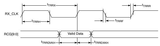
Figure 16. TBI Single-Clock Mode Receive AC Timing Diagram
