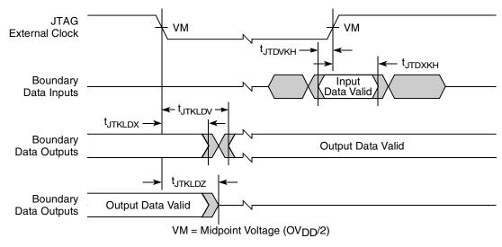
Figure 32. Boundary-Scan Timing Diagram
