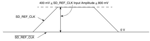
Figure 42. Single-Ended Reference Clock Input DC Requirements
