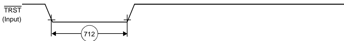
Figure 2-22. \overline{\text{TRST}} Timing Diagram
