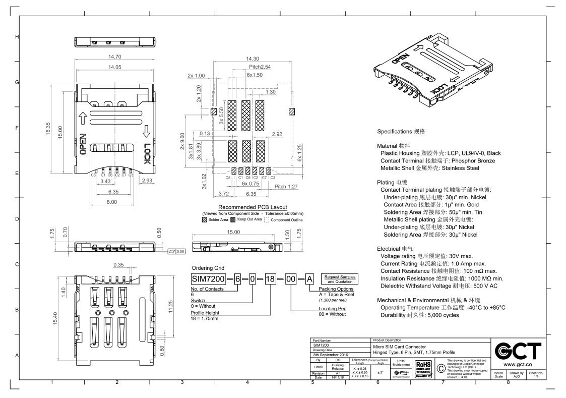
Slide metal lid from 'LOCK' position to 'OPEN' position
