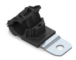
Ratchet P-Clamp, 0.50 - 0.77" Bundle Dia, 180° Short, .41" Hole Dia, PA66HIRHSUV/ST/ZN, Black, 20/bag
