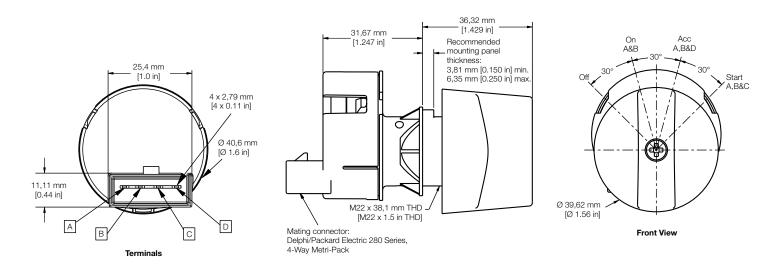
Figure 2. Model 90233 Rotary Switch Dimensions
