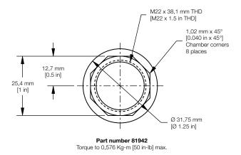
**Figure 8. Mounting Plug Dimensions**
