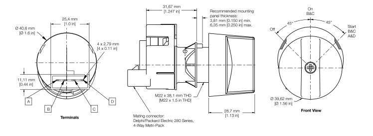
Figure 3. Model 50087487 Rotary Switch Dimensions
