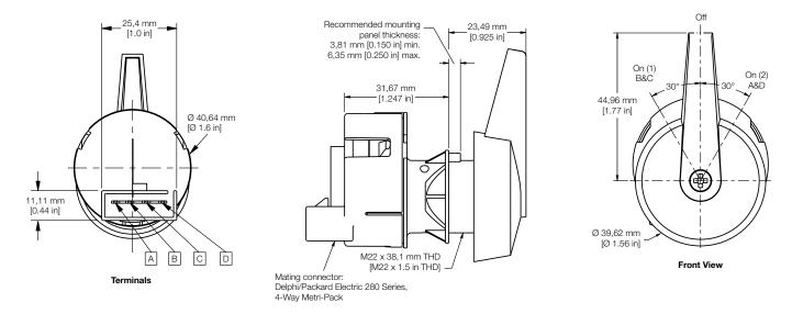
Figure 4. Model 50089737 Rotary Switch Dimensions
