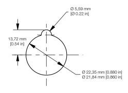
Recommended mounting panel thickness: 3,81 mm [0.15 in] min. 6,35 mm [0.25 in] max.
