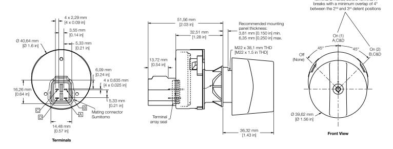
Figure 5. Model 32309969 Rotary Switch Dimensions
