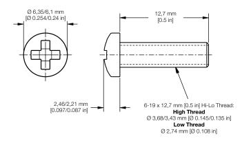
Part number 84833 #6-19 x 12,7 mm [0.5 in] screw Torque to 0,046 Kg-m [4 in-lb]
