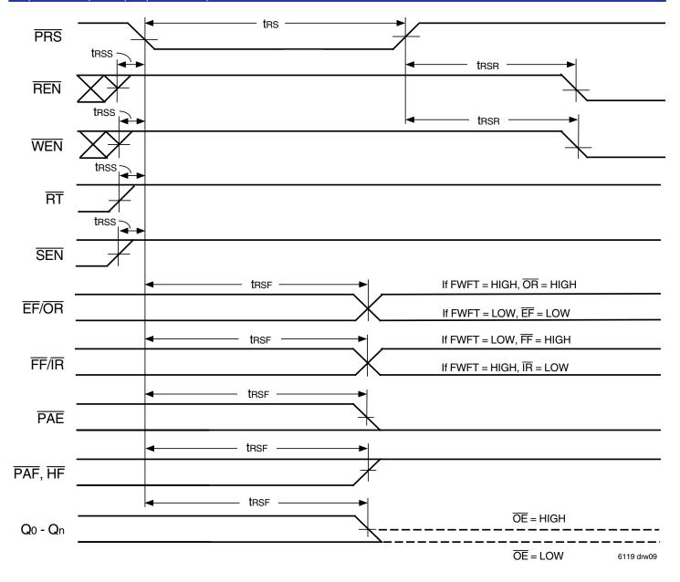
Figure 6. Partial Reset Timing
