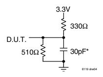
Figure 2a. Output Load
