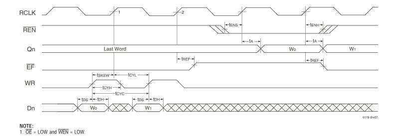
Figure 24. Asynchronous Write, Synchronous Read, Empty Flag Operation (IDT Standard Mode)
