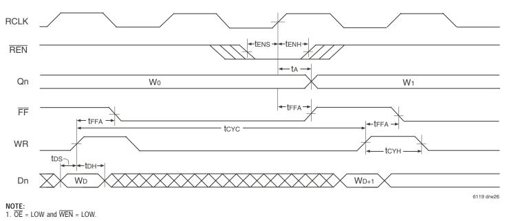
Figure 23. Asynchronous Write, Synchronous Read, Full Flag Operation (IDT Standard Mode)
