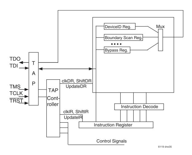
Figure 32. Boundary Scan Architecture
