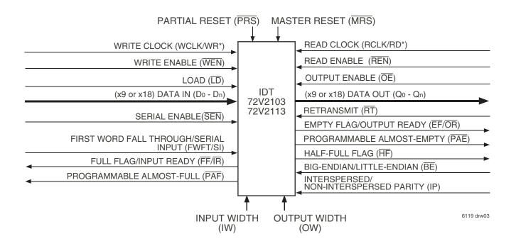
Figure 1. Single Device Configuration Signal Flow Diagram
