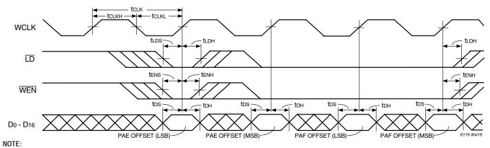
1. This diagram is based on programming the IDT72V2103/72V2113 x18 bus width. Add one extra cycle to both the PAE offset and PAF offset for x9 bus width.
