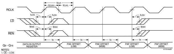
2. This diagram is based on programming the IDT72V2103/72V2113 x18 bus width. Add one extra cycle to both the PAE offset and PAF offset for x9 bus width.
