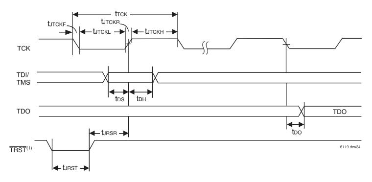
1. During power up, TRST could be driven low or not be used since the JTAG circuit resets automatically. TRST is an optional JTAG reset.
