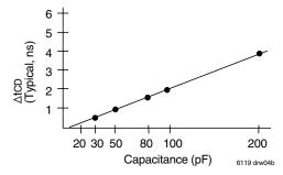
Figure 2c. Lumped Capacitive Load, Typical Derating
