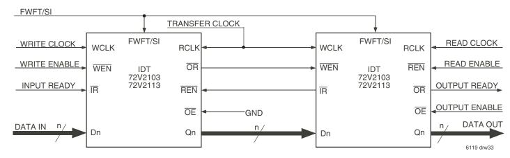
Figure 30. Block Diagram of Depth Expansion
