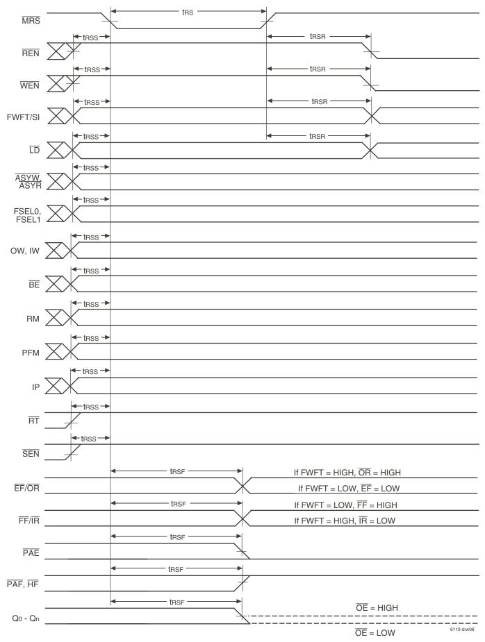
Figure 5. Master Reset Timing
