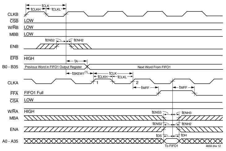
Figure 9. FFA Flag Timing and First Available Write when FIFO1 is Full.
