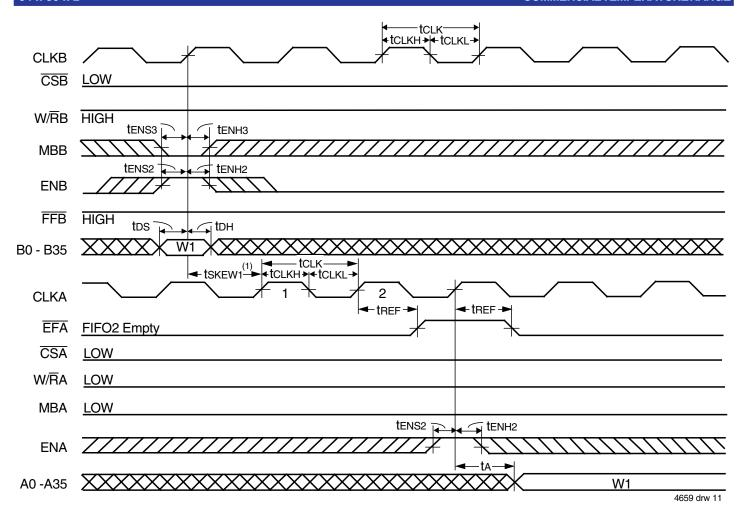
Figure 8. **EFA** Flag Timing and First Data Read when FIFO2 is Empty
