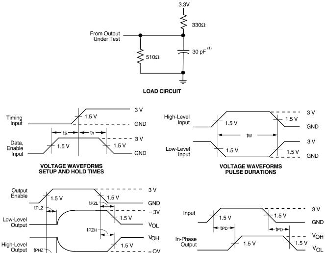
**VOLTAGE WAVEFORMS ENABLE AND DISABLE TIMES**
