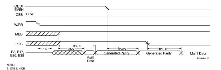
Figure 20. Parity Generation Timing when Reading from Mail1 Register
