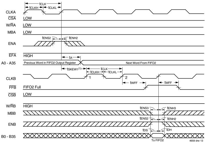
Figure 10. FFB Flag Timing and First Available Write when FIFO2 is Full
