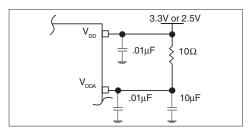
FIGURE 1. POWER SUPPLY FILTERING
