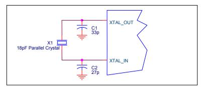
Figure 2. CRYSTAL INPUt INTERFACE
