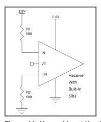
Figure 4A. Unused Input Handling
