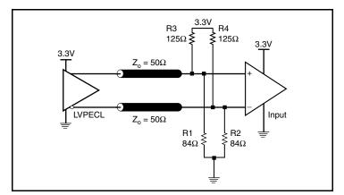
Figure 5B. 3.3V LVPECL Output Termination
