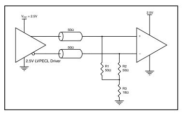
Figure 6B. 2.5V LVPECL Driver Termination Example
