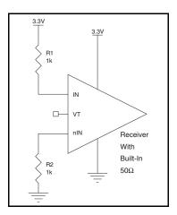
Figure 4B. Unused Input Handling
