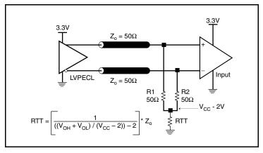
Figure 5A. 3.3V LVPECL Output Termination
