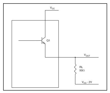
Figure 7. LVPECL Driver Circuit and Termination
