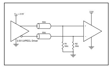
Figure 6C. 2.5V LVPECL Driver Termination Example
