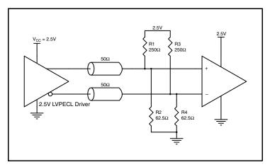
Figure 6A. 2.5V LVPECL Driver Termination Example
