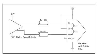
Figure 3C. IN/nIN Input with Built-In 50 $\Omega$  Driven by a CML Driver with Open Collector
