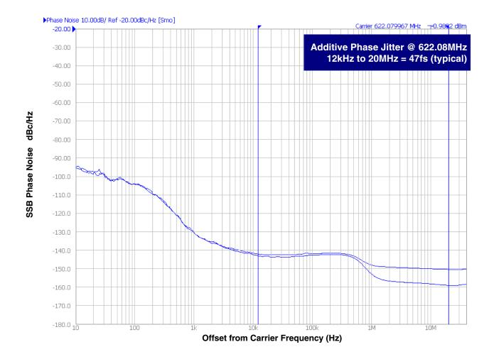
As with most timing specifications, phase noise measurements have issues relating to the limitations of the equipment. Often the noise floor of the equipment is higher than the noise floor of the device. This is illustrated above. The device meets the noise floor of what is
