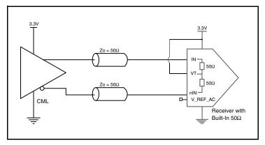
Figure 2C. IN/nIN Input with Built-In 50 $\Omega$  Driven by a CML Driver with Open Collector
