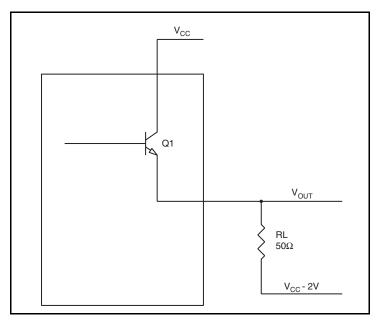
Figure 6. LVPECL Driver Circuit and Termination
