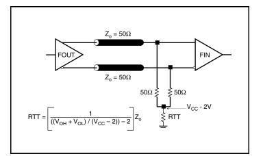
Figure 3A. 3.3V LVPECL Output Termination
