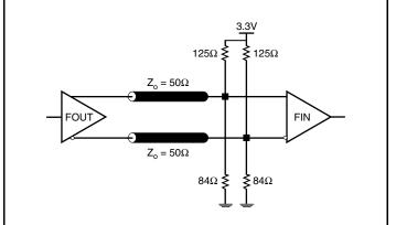
Figure 3B. 3.3V LVPECL Output Termination
