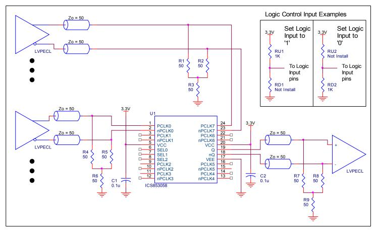
Figure 5. ICS853058 Schematic Example
