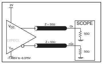
LVPECL Output Load AC Test Circuit
