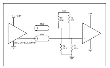
Figure 4A. 2.5V LVPECL Driver Termination Example
