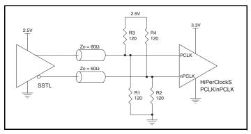
Figure 2E. HiPerClockS PCLK/nPCLK Input Driven by an SSTL Driver
