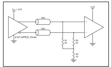
Figure 4B. 2.5V LVPECL Driver Termination Example
