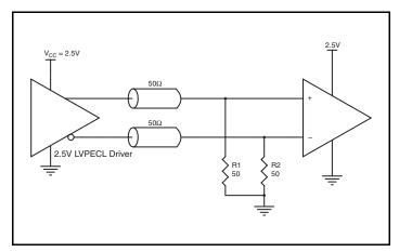
Figure 4C. 2.5V LVPECL Driver Termination Example
