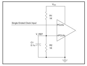
Figure 1. Single-Ended Signal Driving Differential Input
