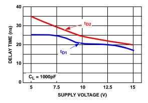
FIGURE 11. PROPAGATION DELAY vs SUPPLY VOLTAGE
