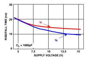
FIGURE 10. RISE/FALL TIME vs SUPPLY VOLTAGE
