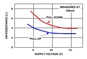
FIGURE 6. ON-RESISTANCE vs SUPPLY VOLTAGE
