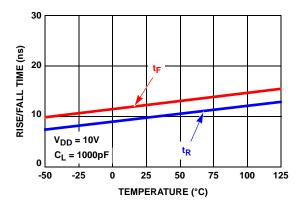
FIGURE 12. RISE/FALL TIME vs TEMPERATURE
