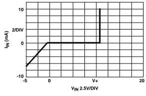
FIGURE 3. INPUT CURRENT vs VOLTAGE
