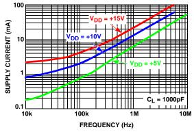
FIGURE 7. AVERAGE SUPPLY CURRENT vs VOLTAGE AND FREQUENCY
