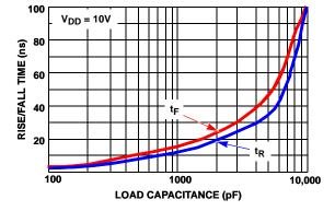
FIGURE 9. RISE/FALL TIME vs LOAD
