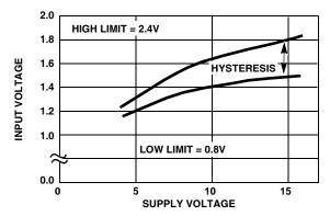
FIGURE 2. SWITCH THRESHOLD vs SUPPLY VOLTAGE
