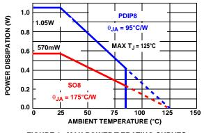
FIGURE 1. MAX POWER/DERATING CURVES
