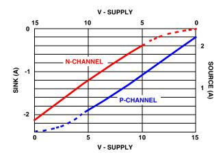
FIGURE 4. PEAK DRIVE vs SUPPLY VOLTAGE
