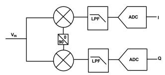
FIGURE 4. I AND Q PROCESSING OF THE SIGNAL
