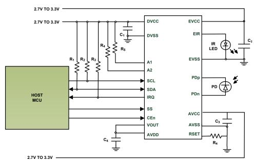
FIGURE 1. APPLICATION DIAGRAM
