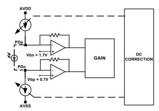
FIGURE 7. CONNECTING PD TO AFE
