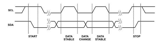
FIGURE 11. VALID DATA CHANGES, START AND STOP CONDITIONS
