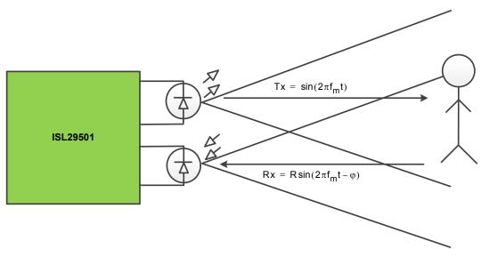
FIGURE 3. TRANSMITTED AND RECEIVED SIGNAL IN A SYSTEM
