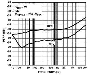
FIGURE 22. PSRR vs FREQUENCY
