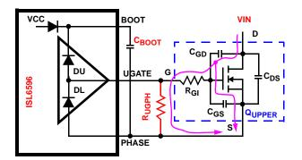
FIGURE 5. GATE TO SOURCE RESISTOR TO REDUCE UPPER MOSFET MILLER COUPLING
