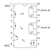
1. (N/C) 2. + LED - Form A Relay #1 3. - LED - Form A Relay #1 4. + LED - Form A Relay #2 5. - LED - Form A Relay #2 6. Emitter - Phototransistor 7. Collector - Phototransistor 8. (N/C) 9. LED - Phototransistor +/-10. LED - Phototransistor -/+ 11. Output - Form A Relay #2 12. Common Source Relay #2 13. Output - Form A Relay #2 14. Output - Form A Relay #1 15. Common Source Relay #1 16. Output - Form A Relay #1
