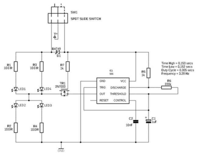
The circuit has two operating modes. Flashing LED and constant illumination LED. This is determined by the position of the switch.
