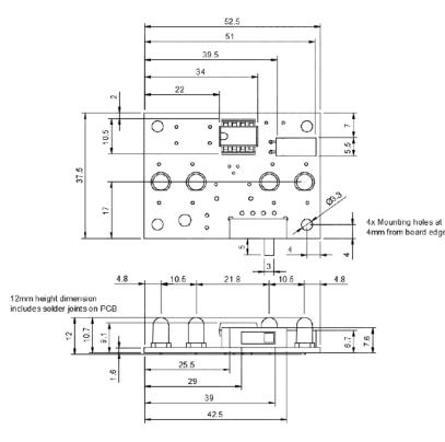
All dimensions are in mm. The PCB has four mounting holes 3.3mm in diameter. These holes are 4mm from the board edge
